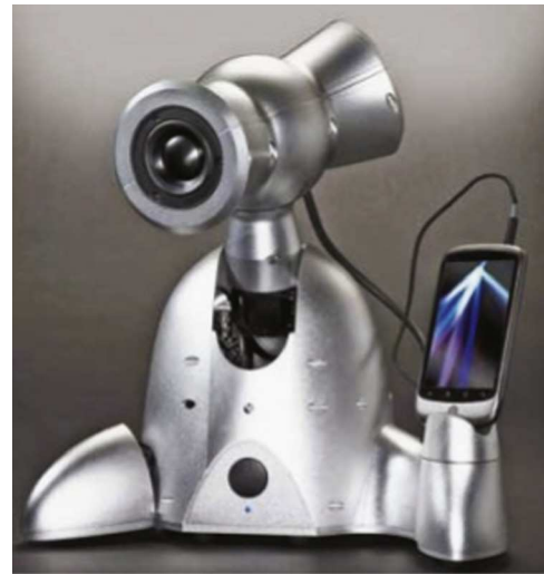
Fig. 1. Shimi is a faceless, five DoF, smart phone powered, robotic speaker dock which uses musical intelligence to engage users and dance to music. Shimi has five DoFs: three in its head, one on the hand that holds the phone, and one on its foot for tapping.
